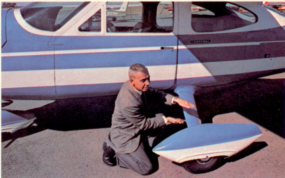
Cardinal's unique landing gear fairing improves appearance and reduces drag. It conceals a new one-piece tubular spring steel landing gear.
